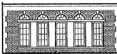
Arched windows with brick corbeling
