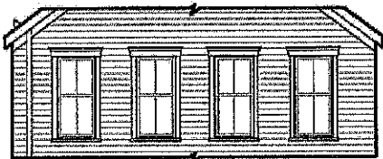
Flat trim with multiple window units
