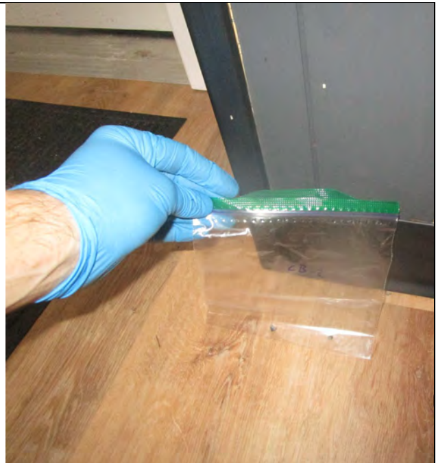
View of sample CB-2: Black cove base in coffee shop. No asbestos detected.
