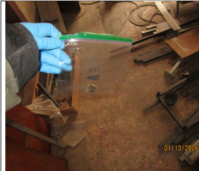
View of sample FS-3: Sheet flooring on second floor of 532 K. No asbestos detected.
