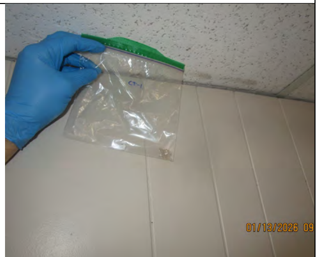
View of sample CT-1: Suspended ceiling tile in consignment shop. No asbestos detected.
