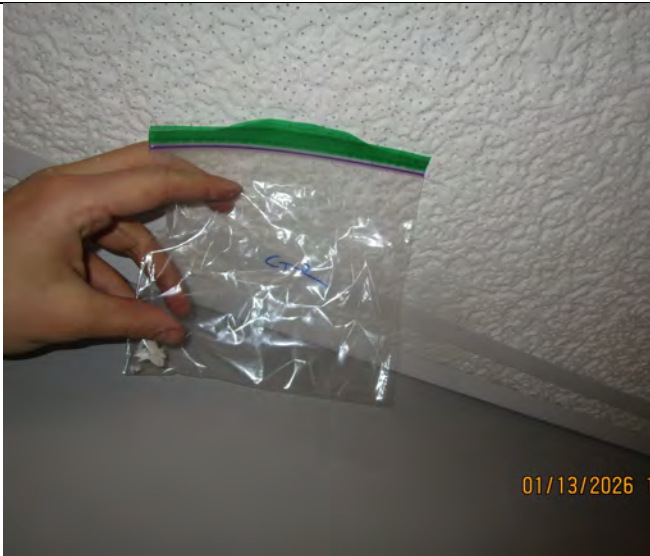
View of sample CT-1: 2x2 pinhole ceiling tile in 1 st floor. No asbestos detected.
