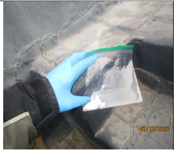
View of sample RM-1: Black roof membrane. No asbestos detected.
