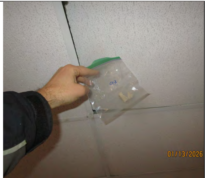
View of sample CT-3: 2x4 ceiling tile on second floor. No asbestos detected.
